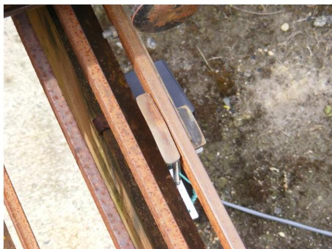
The micro switch activated by the locomotive
