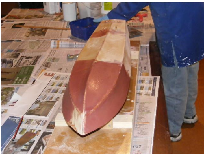
The hull after the application of mico balloons
